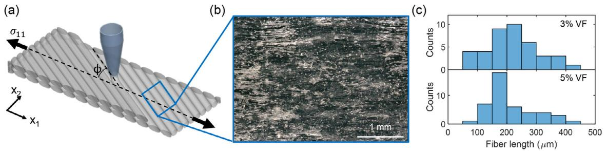
**Fig. 1.** (a) Schematic of the direct ink writing process. The angle  $\phi$  indicates the angle between the loading direction and the predominant fiber orientation. (b) Representative optical image showing aligned fibers in the printed sample. (c) Fiber length distribution for 3% and 5% volume fraction samples.
